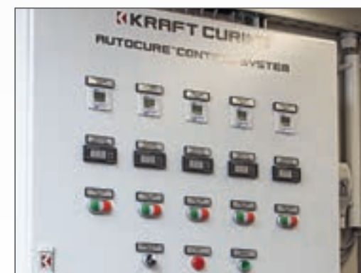
Automatic controls provide for unsupervised production and consistent results without over-heating the concrete.
