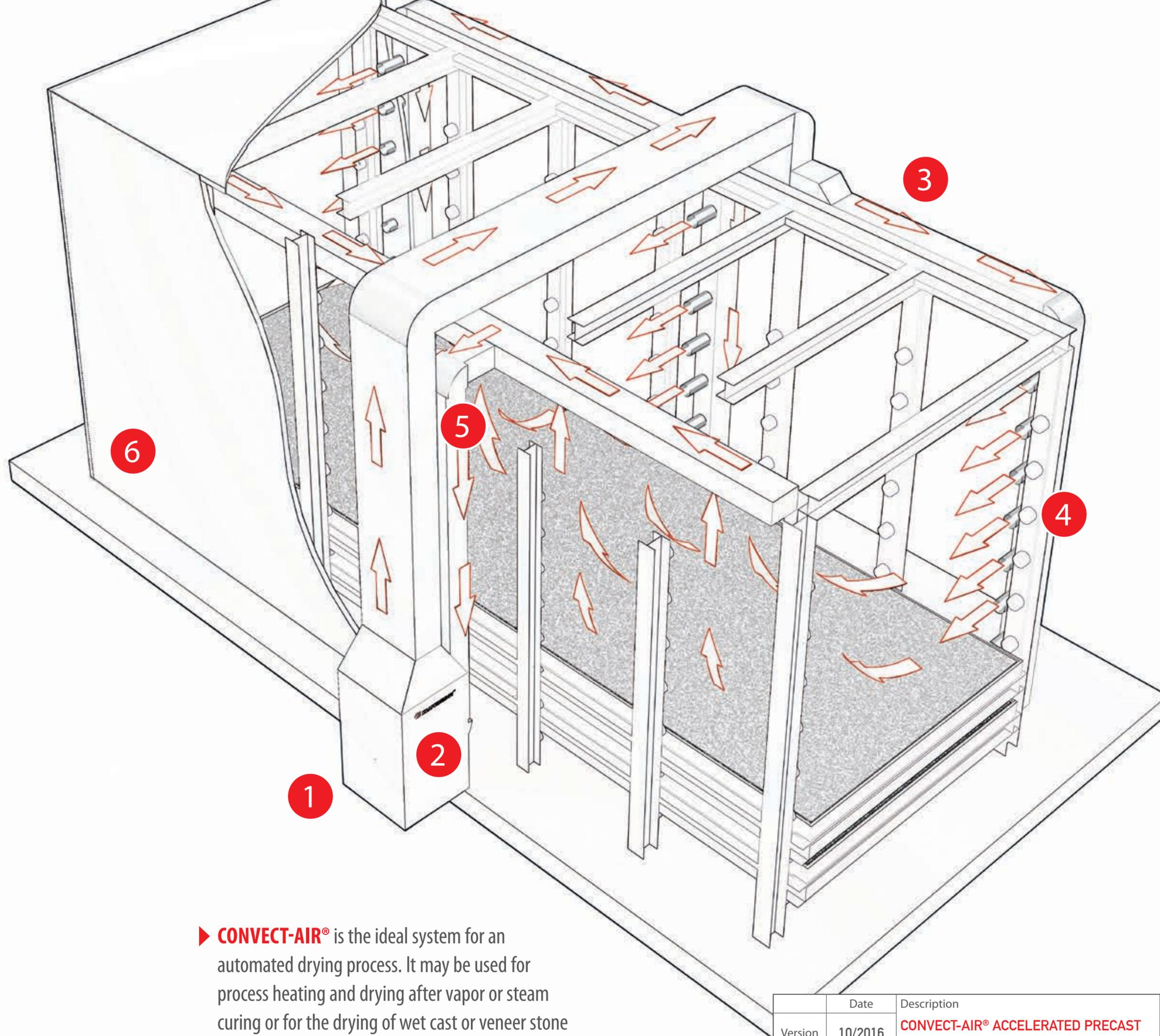
► **CONVECT-AIR®** is the ideal system for an automated drying process. It may be used for process heating and drying after vapor or steam curing or for the drying of wet cast or veneer stone products where residual moisture may create quality issues.
