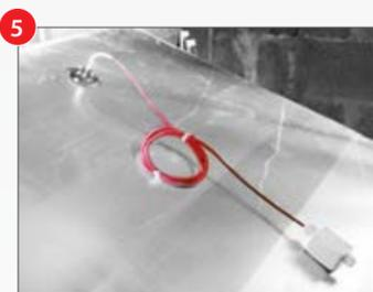
A thermostat is located in the distribution manifold. Once the desired curing temperature is reached, the heater switches off. It turns on again to maintain temperature when fresh concrete products are introduced. The circulation ventilator operates continuously throughout operation to maintain even temperature.
