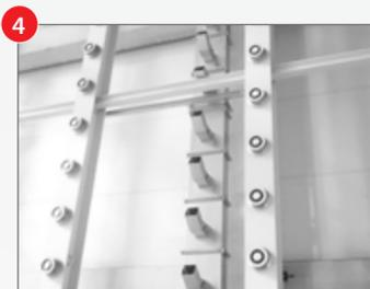
Vertical air supply ducts inside the curing chamber provide for consistent temperature and low air speed. The location and direction of the air supply outlets prevent accelerated evaporation of moisture from the concrete surface.
